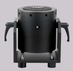
DynaLabs permanent magnet shakers create motion by magnets and coils pushing and pulling each other, similar to the technology used in loudspeakers. The PM-101 shaker is identical to the PM-100, except it does not include an integrated amplifier. For those requiring an amplifier, the SA-400 and SA-500 models are available. With its lightweight design and powerful performance, it is the ideal solution for modal and vibration testing.
