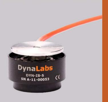
Depending on the structure's dimensions and the desired excitation frequencies and levels, either modal shakers or inertial shakers may be used for vibration testing. Compared to the modal shakers, the connection styles are different. The body of the inertial shaker itself vibrates. For this reason, inertial shakers are fixed directly to the structure. Compared to modal shakers, it is easier to use. DynaLabs inertial shakers are easily mounted and highly portable. They can be used as hand-held.
