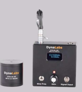
Depending on the structure's dimensions and the desired excitation frequencies and levels, either modal shakers or inertial shakers may be used for vibration testing. Compared to the modal shakers, the connection styles are different. The body of the inertial shaker itself vibrates. For this reason, inertial shakers are fixed directly to the structure. Compared to modal shakers, it is easier to use. DynaLabs inertial shakers are easily mounted and highly portable. They can be used as hand-held.
